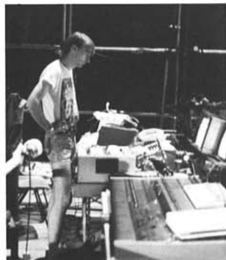
Follow spot operator Peter Hart in the lighting control area at Battersea. The Celco memory lighting control desk in the foreground was used for the BBC1 television performance, with BBC monitors in picture, right centre. The two Berkey Colortrack controls for performance lighting are furthest from camera.
