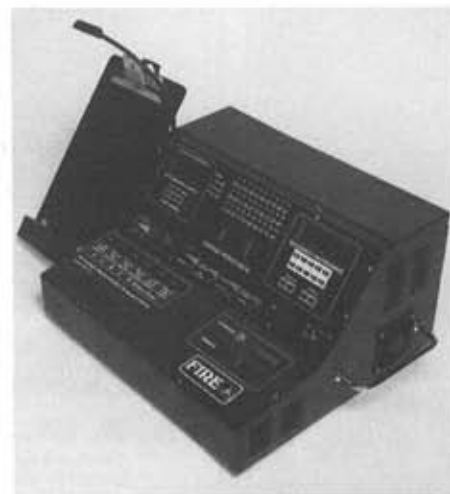
Le Maitre's custom-built 30-way firing system.
