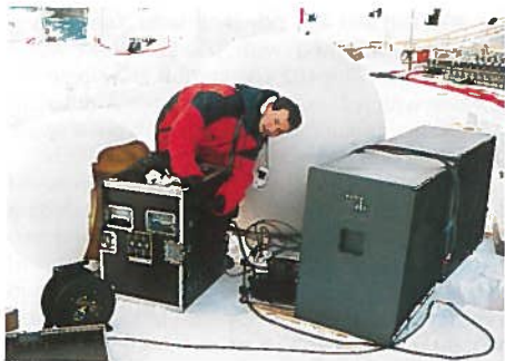
Fake snowballs are fitted with JBL infills, subs and Lab Gruppen amps ready to blend seamlessly (well almost) into the background, whilst below, the sub zero temperatures take their toll.
