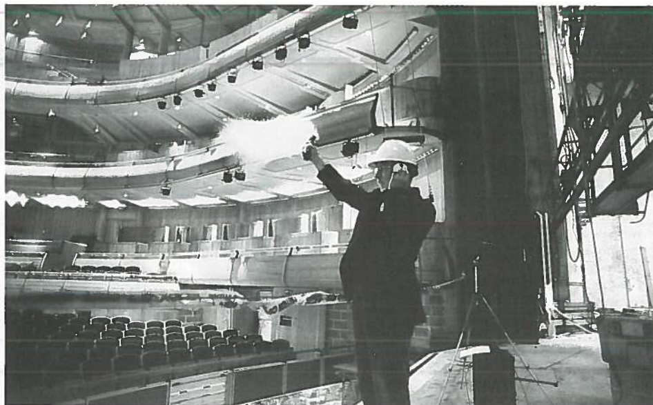
Derek Sugden of Arup Acoustics fires a starting pistol to test the acoustics of the new auditorium, December 1993. photo: Richard Davies
