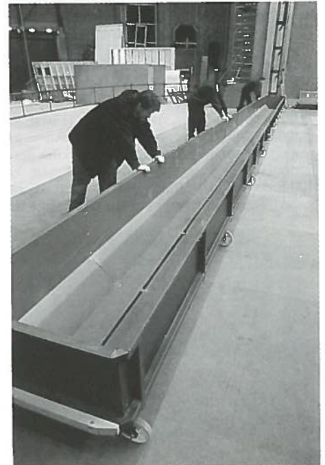
The below stage cloth storage bin racks.
