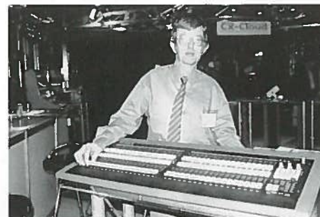
Iain Price-Smith of Multiform with the Zodiac 36, a 36 channel level memory lighting desk that stores fade times as well as levels for each scene in a memory. It also has pause/override facilities, LTP operation and 0-10V/DMX/MIDI outputs.
