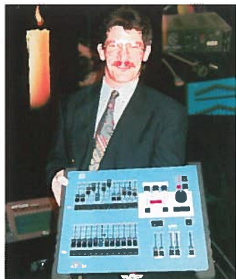
Gary Pritchard of LSC with the prototype of the Axiom Atom lighting desk, available in 12/24 and 24/48 versions. Each sub masters can control pre-recorded scenes or chases, and the desk has nine pages of memory.
