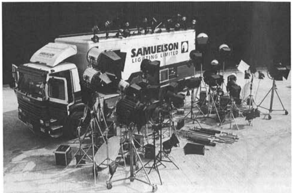
A Samuelson Lighting 60kW equipment carrying mobile alternator pictured outside the new Stage 1 at Bray Studios in Berkshire with a full complement of luminaires, accessories, and distribution equipment.
