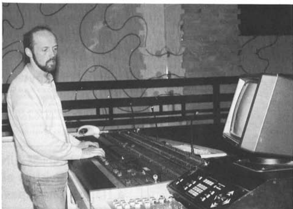
Fried Buttstedt of Flashlight pictured at the Celco Series 2 90 channel control desk, located on the balcony control area. To the right is the Coemar Robot controller.
