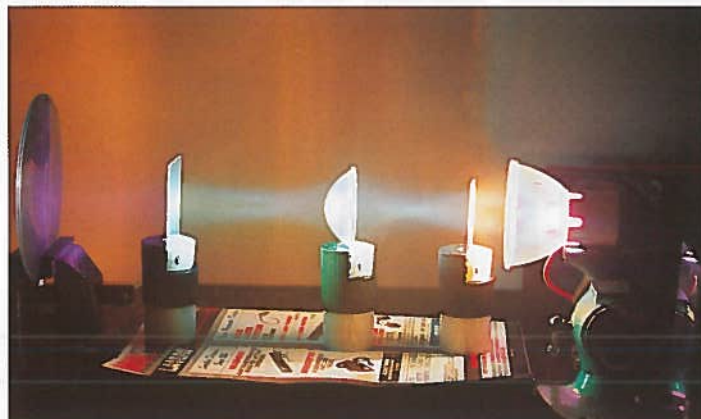
Early workbench tests of dichroic filters and the metal halide light source used to develop the optical configurations of the first Vari-Lite prototype.
