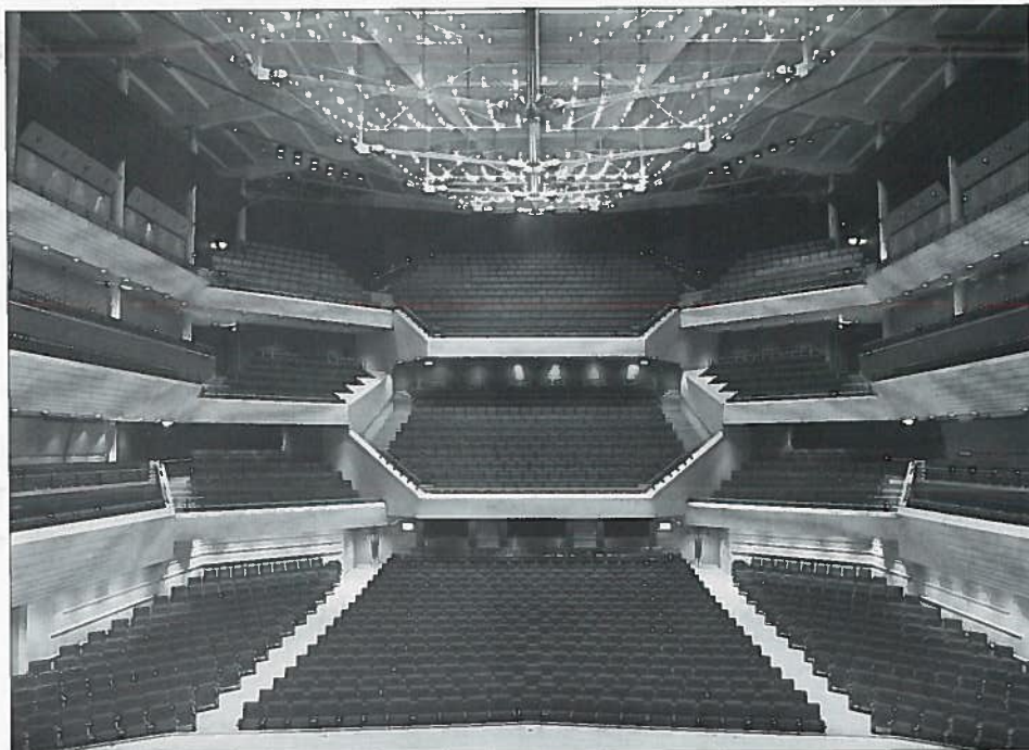
The auditorium accommodates a seated audience of 2,400. With very few exceptions, all seats have a grille panel in the floor that covers both A/C and heat supplies which not only ensures comfort, but also provides a uniformity of temperature throughout the hall.
