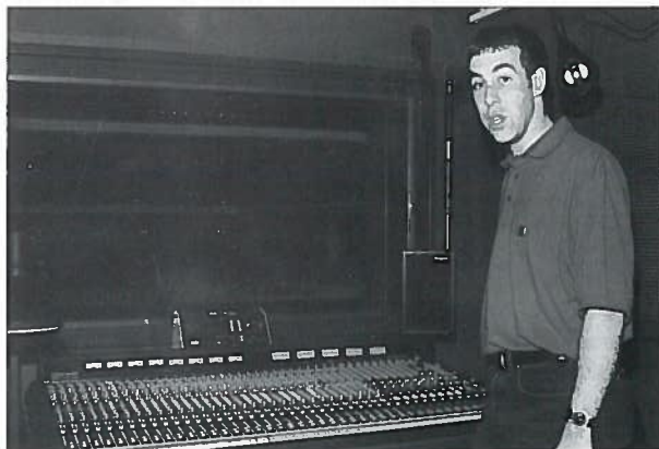
Technical manager Chris Wright with the Century Vx console. Originally specified as a 24-channel desk, this was upgraded to 32 channels at the request of the BBC.
