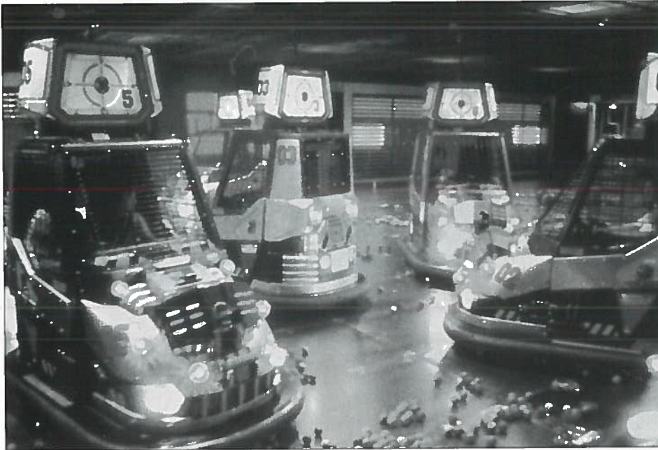
On the Mad Bazoooka ride at Segaworld, competitors in Hyper Battle Carts blast each other with machine cannons that fire balls at 90mph. Enclosed within 30 tonnes of steel, the Mad Bazoooka uses some 30 fibre optic sensors connected by 250m of cabling just to keep score.
