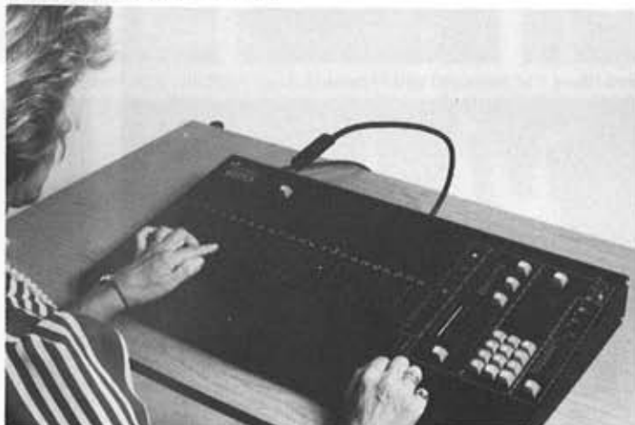
'Action' - Strand's exciting new single scene lighting control with basic memory and effects.
