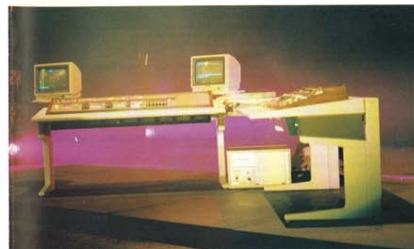
- Strand Lighting's top-of-the-range memory lighting control - is a customised modular system 999 channels and 1536 dimmers. Studio and theatre versions are available, with up to 20 pres with flash and inhibit facilities, advanced special effects, and a pan/tilt/focus control.
