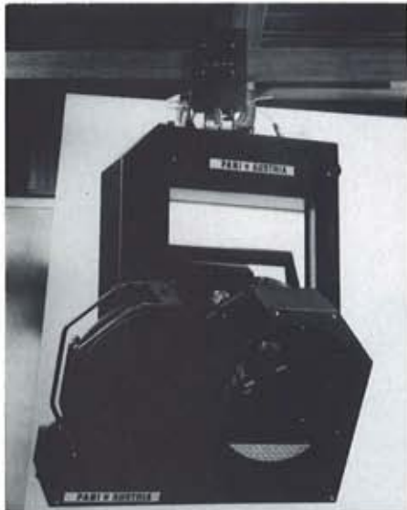
A parabolic 1001 low voltage beamlight in a motorised PEF-M unit and with a colour change mechanism - Theater an der Wien. Below: control unit for the PEF-M system.
