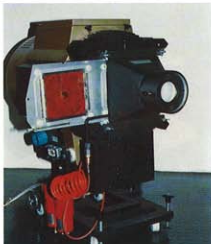
Backstage at the Staatsoper, Vienna, and the shadow projection system used to produce the 'ship' in a seventies production of The Flying Dutchman - designer Günther Schneider-Siemssen. The ballast unit is on wheels in the centre of the main picture. A 6½k Xenon unit had specially built shutters to fade the light source, and an old Pani 5k (left) with a double drive effect unit was used to produce 'waves'. In case of emergency an old Pani 10k tungsten halogen projector awaits its call (extreme right). The smaller picture shows a close-up of the track system for the model ship.
