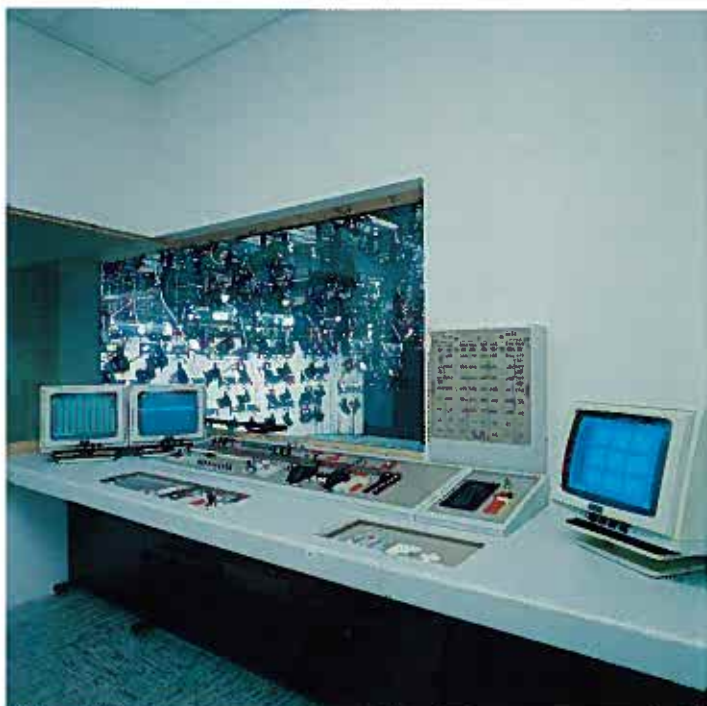
Galaxy II lighting console with memory back-up (left) and PALS control (right).
