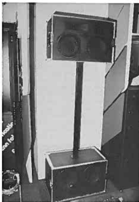
This unusual loudspeaker combination is manufactured by Leech. The two units are flight cased clipped together face-to-face.
