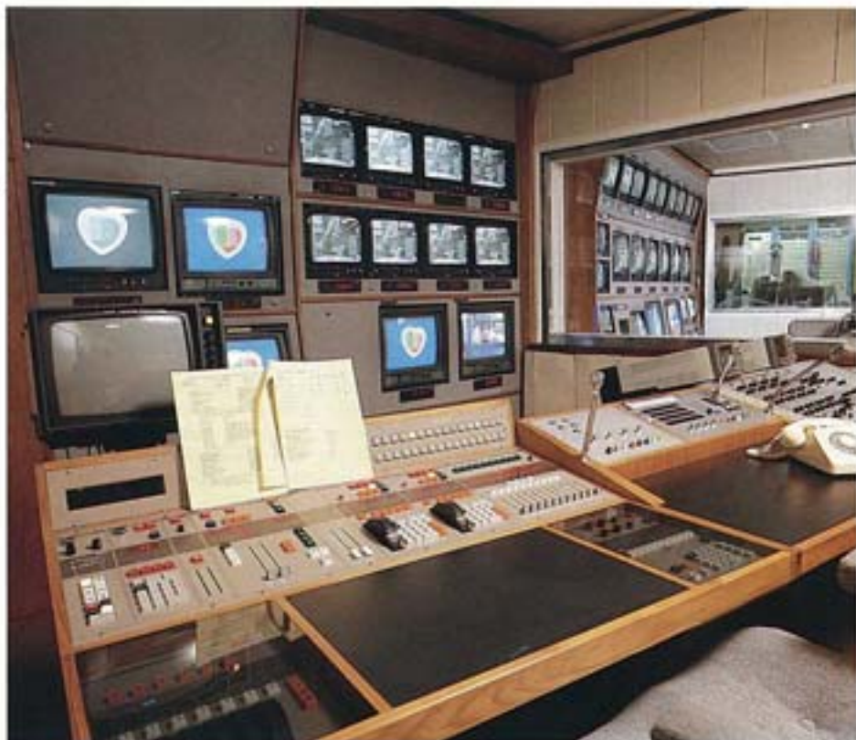
One of two Strand Galaxy lighting control systems recently installed at the South Bank Studios of London Weekend Television. Other Galaxies have been supplied within the last few months to the BBC for Elstree and Cardiff and to Yorkshire Television in Leeds and TVS at Southampton.
