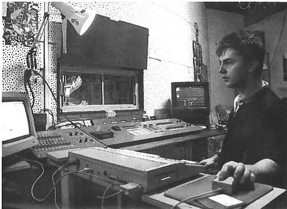
Nicky Rintoul, assistant electrician at the theatre, operating the Arri Imagination 250 lighting board with backup (centre) and the Atari 1040 computer (left).
