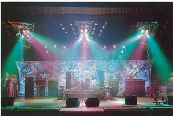
In order to make the rig as versatile as possible, 21 of the 100 par lamps were fitted with colour changers.
