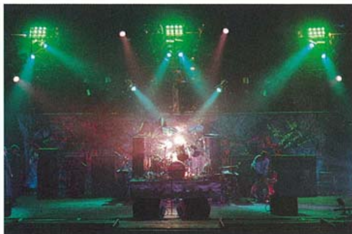
The rig features three Genie Superlifts fronted by Expanet grilles which create a diffused effect.
