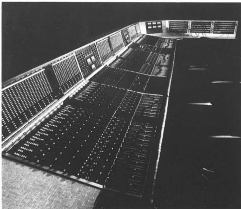
The 60 channel 32 group film post production console built for Pinewood Studios and commissioned in September 1981. In its day it was the largest automated console in the world.
