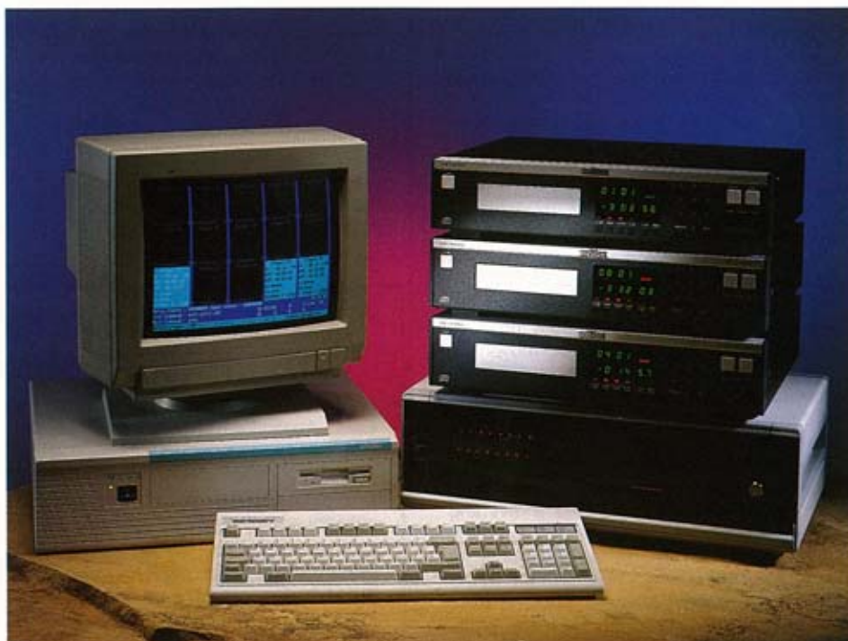
The FX system: a PC-based hardware/software package that can operate up to 15 CD221s.
