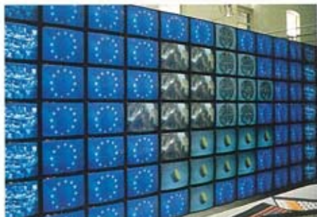
Imagination's Videowall at Expo 92 which featured 98 TV monitors, six video sources and a frame accurate matrix switcher.
